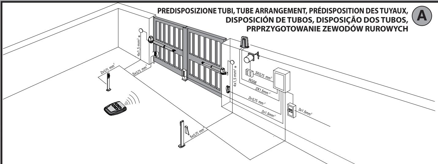
SCHEMA D'INSTALLAZIONE-INSTALLATION DIAGRAM-SCHÉMA D'INSTALLATION
