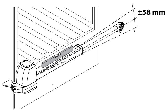
CORRETTA INSTALLAZIONE - CORRECT INSTALLATION
